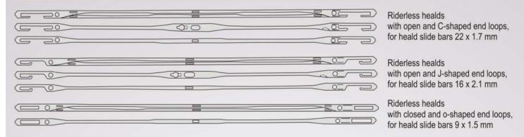
Varieties of the Healds: Simplex type is offered in standard Strips thickness of 5.5mm x 0.3mm / 0.38mm & Duplex 6mm x 0.3mm / 0.25mm & 7.2mm x 0.3mm / 0.25mm to suit the finer & courser yarn. Our Automatic production line allows production of Riderless Healds in the length of 280mm (11") to 457mm (18").
